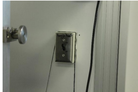
16) Switch off the Rough Pump.
