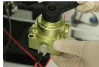
17) Turn handle for HighVac to the Open position.
