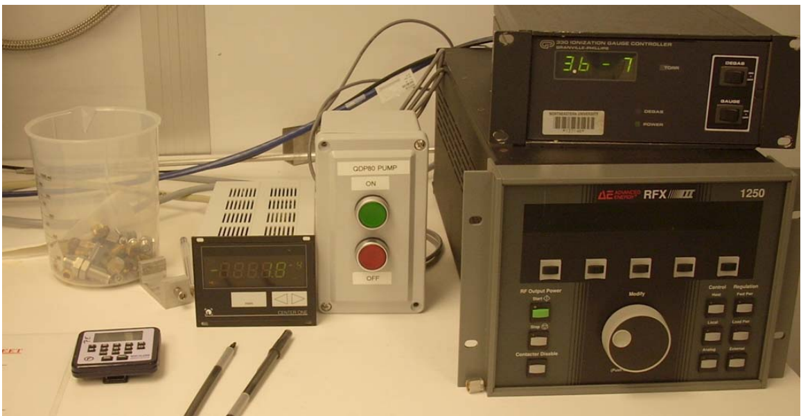
Figure 2 Rough Pump Switch
