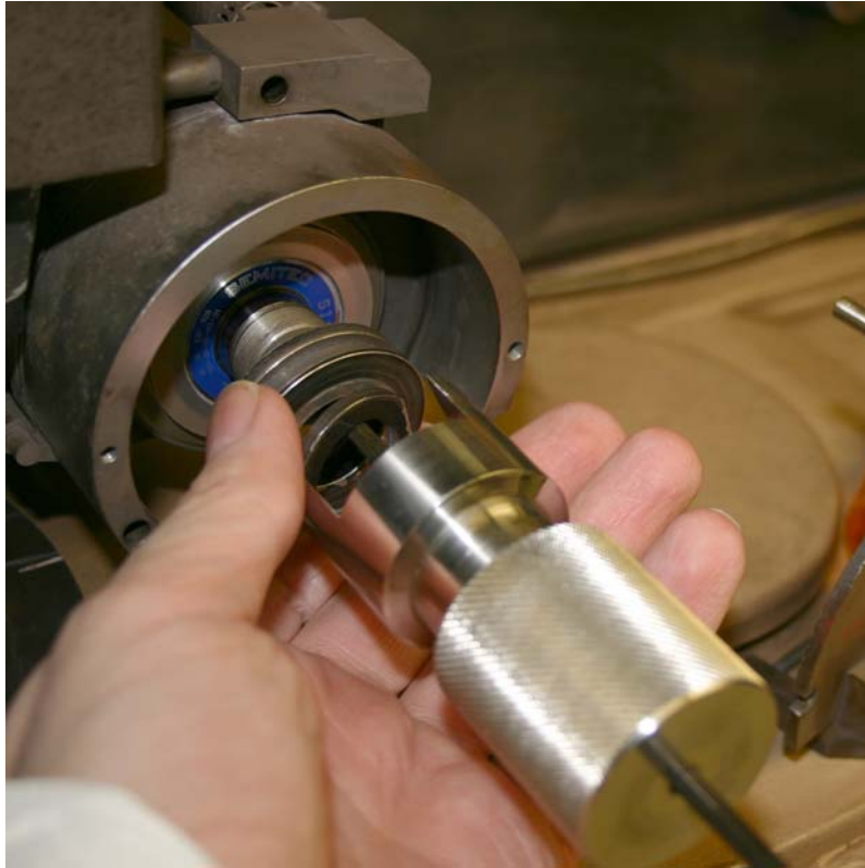
Figure 5. A quick twist CC and the hub bolt and washer are removed exposing the blade
