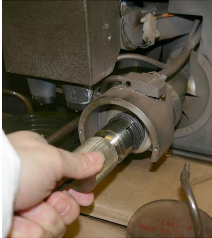
Figure 4. Insertion of hub bolt removal tool
