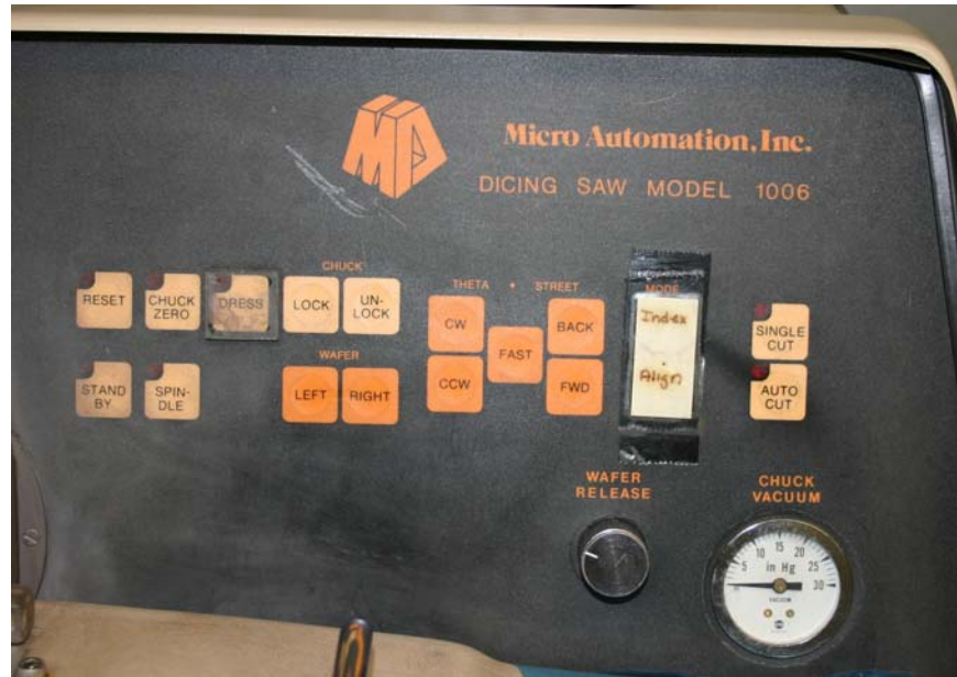
Figure 10 Secondary control panel for alignment and dicing start
