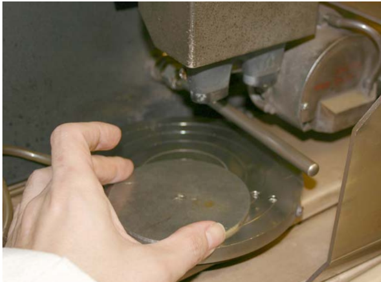
Figure 9. Setting the ref. plate down in the center of the chuck.
