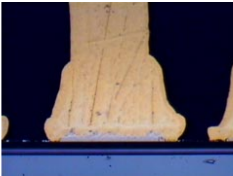
Formation of intermetallic compound
